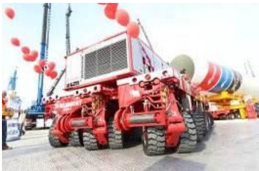
All good things come in threes: 6-axle SPMT with coupled 6-axle SPMT Split and Power Packs on the loading area
